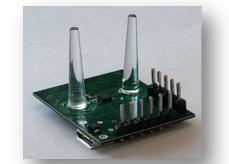
Enable light pipe as 24GHz antenna
