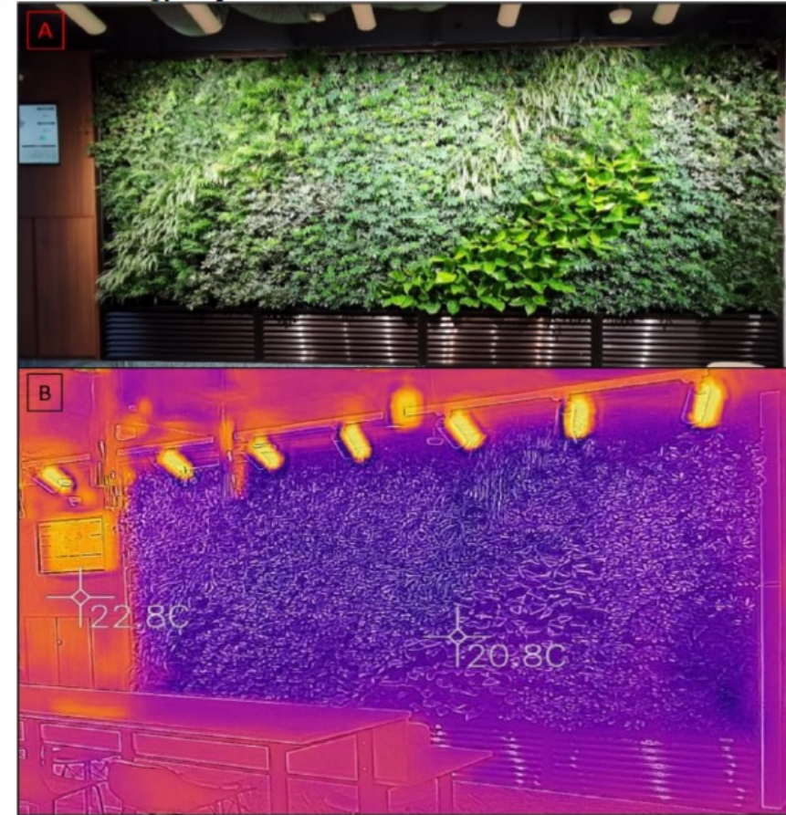
Figure 2: Bravolinear EnvoyAir Active Green wall thermal regulation imaging (B). Source: Used with permission of Bravolinear Tech Limited.
