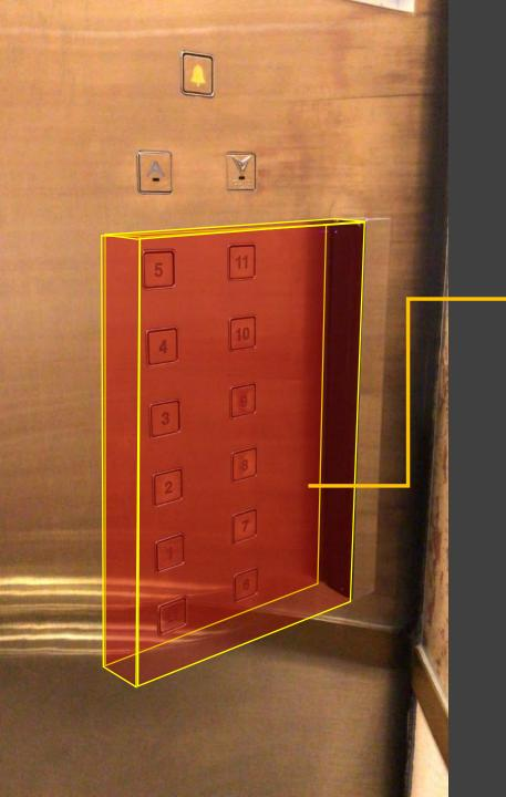
kNOw Touch is made of a 2D infrared distance sensor, providing additional electronic signals to the elevator button panel.
