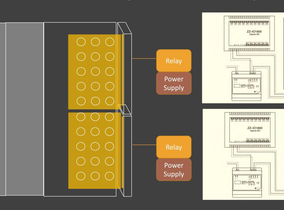
For the case II more-than-16-buttons, two kNOw Touch devices can be connected to two relays separately.
